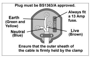
• The YELLOW AND GREEN wire must be connected to the terminal which is marked E \_\_\_\_\_ or coloured green.
